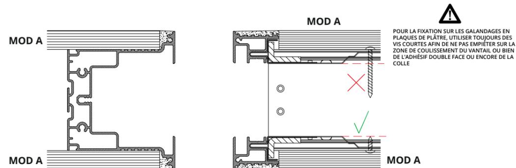
MONTAGE AVEC ESSENTIAL / TECHZERO / MAGNIFICO FIT / 125 PLÂTRE
